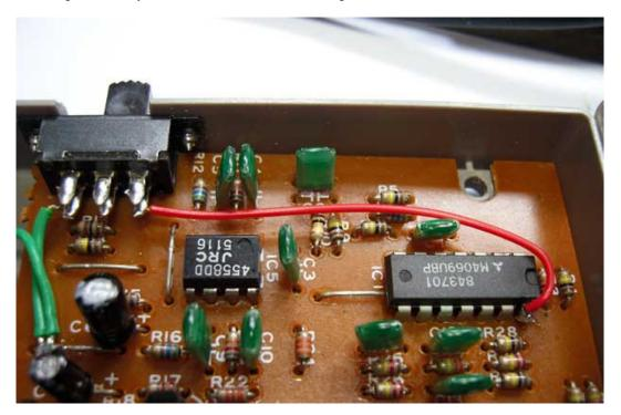
Now you need to install the clock wiring. In order to do this you first have to disconnect the standard internal clock.
