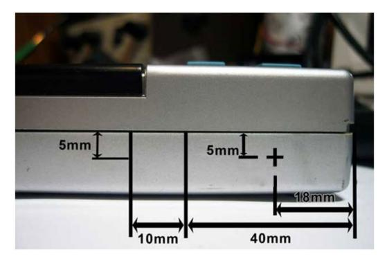
This may not make sense immediately but read on and everything will become clear. The 5mm measurements are from the outer edge / lip of the lower casing as shown, not from the top of the inner lip of the casing edge.
