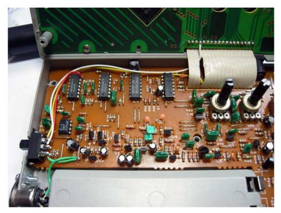
Heres where the wire colours start to matter. Find your DIN-sync interface board and place it where you want it on the voice board. Theres a nice big gap with very few components in the middle of the board but you may have to bend some capacitors out of the way. Be careful that they don't short to other components if you do. The red, yellow and orange wire should be sticking out of the right hand side towards the tempo and volume pots etc.
