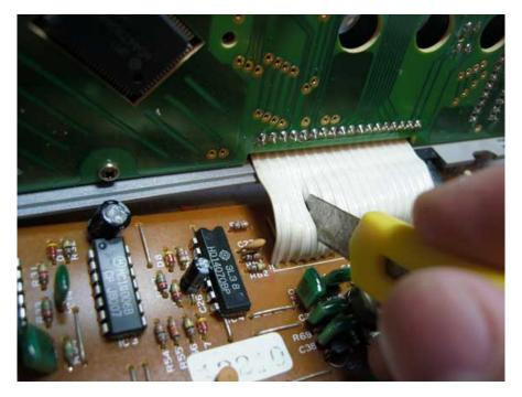
Once you have the fourth wire free of the ribbon cable on either side you can bend it outwards and use a pair of wire cutters to disconnect it.
