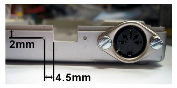
The holes for the mounting screws can then be drilled using the dimensions above. We use a 2mm drill bit for this, but the positioning needs to be as accurate as you can make it., If you haven't cut the slot exactly 10mm wide then it might be better to measure 19mm between the screw hole centres, rather than measure in relation to the slot edge.
