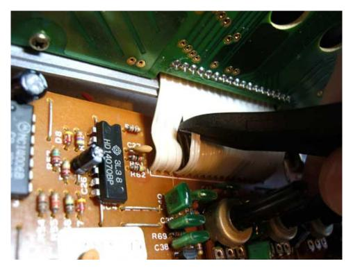
Cut out some of the remaining wire and you should be left with something like the image below. We haven't done it here, but we would recommend leaving a small length of the bare wire sticking out of the voice board as you will need to solder to it next.
