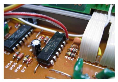
The remaining pair of orange and yellow wires are the play and stop controls and should be wired to the two points on the cpu board (in the top half of the case) as shown below. Orange solders to the left and yellow to the right.
