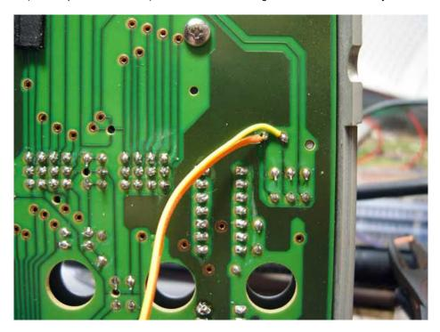
Now solder the green wire from the left hand side of the interface, to the same ground point you used earlier i.e. the jumper next to C6. The white wire should be soldered to the bottom middle pin of the switch, while the blue wire should be soldered to the remining switch pin on the top left. See the wiring diagram at the end of the guide for more details. The switch should now look something like this.
